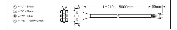
If rotation of rotor is wrong: switch the "V" (black) and "W" (blue) cable to change motor direction.
