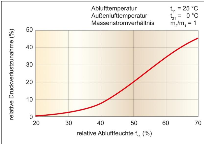
Diagram 2: Pressure loss increase with condensation
