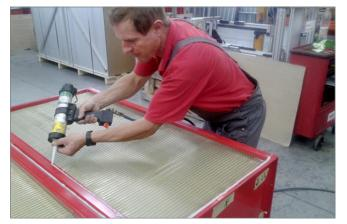
Bild 5: Apply sealing compound
