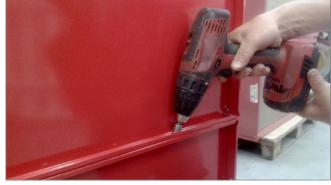
Bild 6: Screw the side wall flanges to one another
