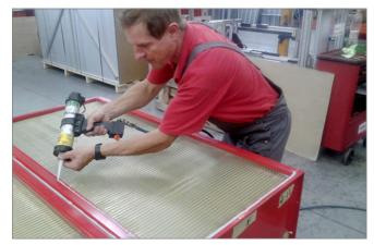
Bild 5: Apply sealing compound
