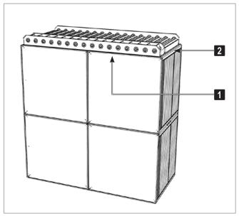
1 Side wall flange with positioning holes
