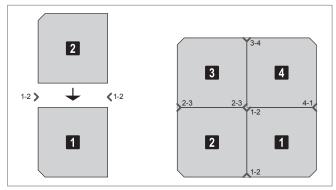
Bild 4: Installation sequence and position of the angle brackets
