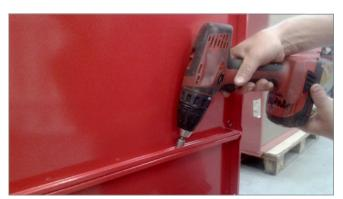
Bild 6: Screw the side wall flanges to one another
