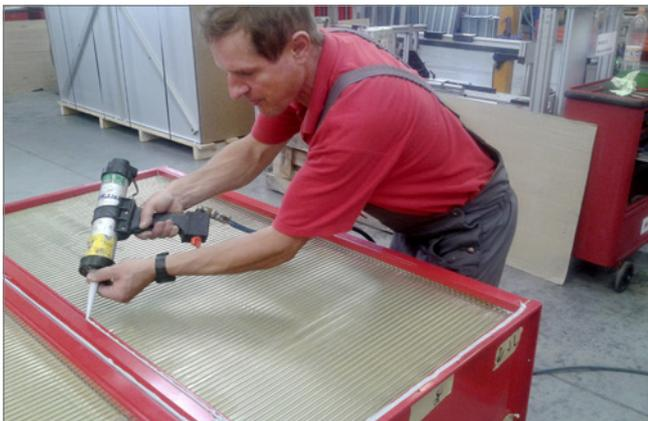
Bild 5: Apply sealing compound
