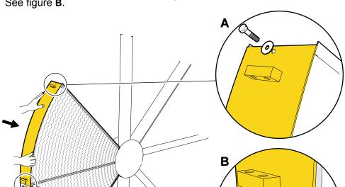
• Fasten the periphery plates together with a clamp bolt. Do not tighten.
