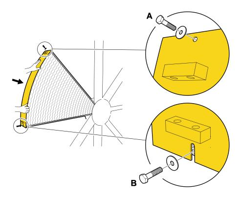
The bolts are tightened when the adjacent periphery plate has been installed.
