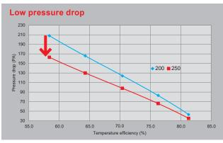
At the same heat recovery efficiency value, the pressure drop is lower in the case of the 250 mm series (red).
