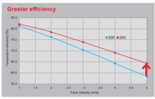
Significantly increased heat recovery efficiency in the case of the 250 mm series (red) in comparison to the standard design.
